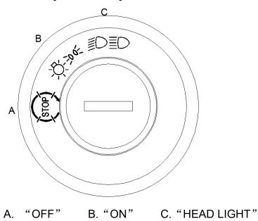
"OFF": Turn the key to this position to stop the engine, switch off all the electrical circuits and remove the key.
