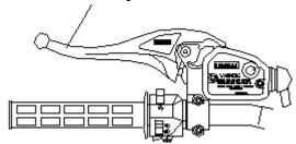
Your ATV has an auxiliary brake provided brakeas a safety feature. It is located on the left handlebar and is operated by the left hand. It is intended as a backup to the main brake system, especially if the main system becomes inoperative.
